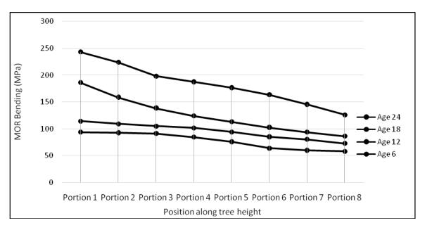
Figure 4: The modulus of rupture on bending tests at different age-group of cultivated *C.* manan at portions height 1 to 8.
