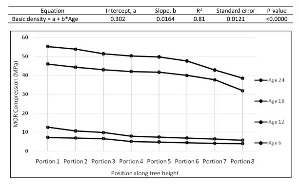
Figure 3: The modulus of rupture on compression tests at various age-group of cultivated *C. manan* at portions height 1 to 8
