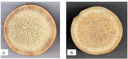
Figure 1: The cross-section is showing a distinct variation in density between an outer and inner part of cultivated 24 years-old (picture A) and a 12 year-old *C. manan.*
